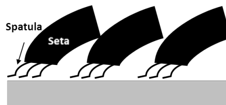
Fig.2: Hierarchical curved beam model.
