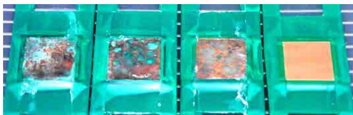
Fig.2 Cu substrates after salt water spraying test for 2000 h (Cu, SiO_2 film/Cu, C_{10} -hybrid film/Cu, and C_{10} -TTA hybrid film/Cu).
