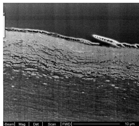
Fig.4 A photograph of a cross section of iron-sulfide coated scale. White area at the surface shows iron-sulfide crystal and black area shows a proteinaceous layer.
