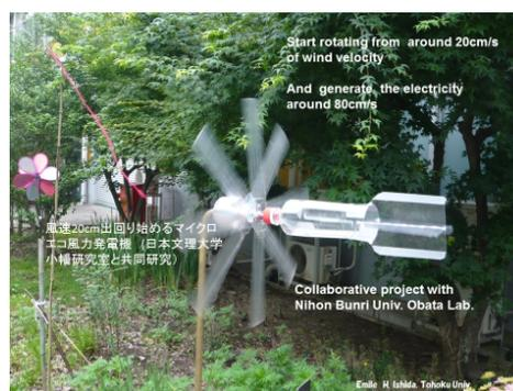
Fig.2 Developed Wind Generator
